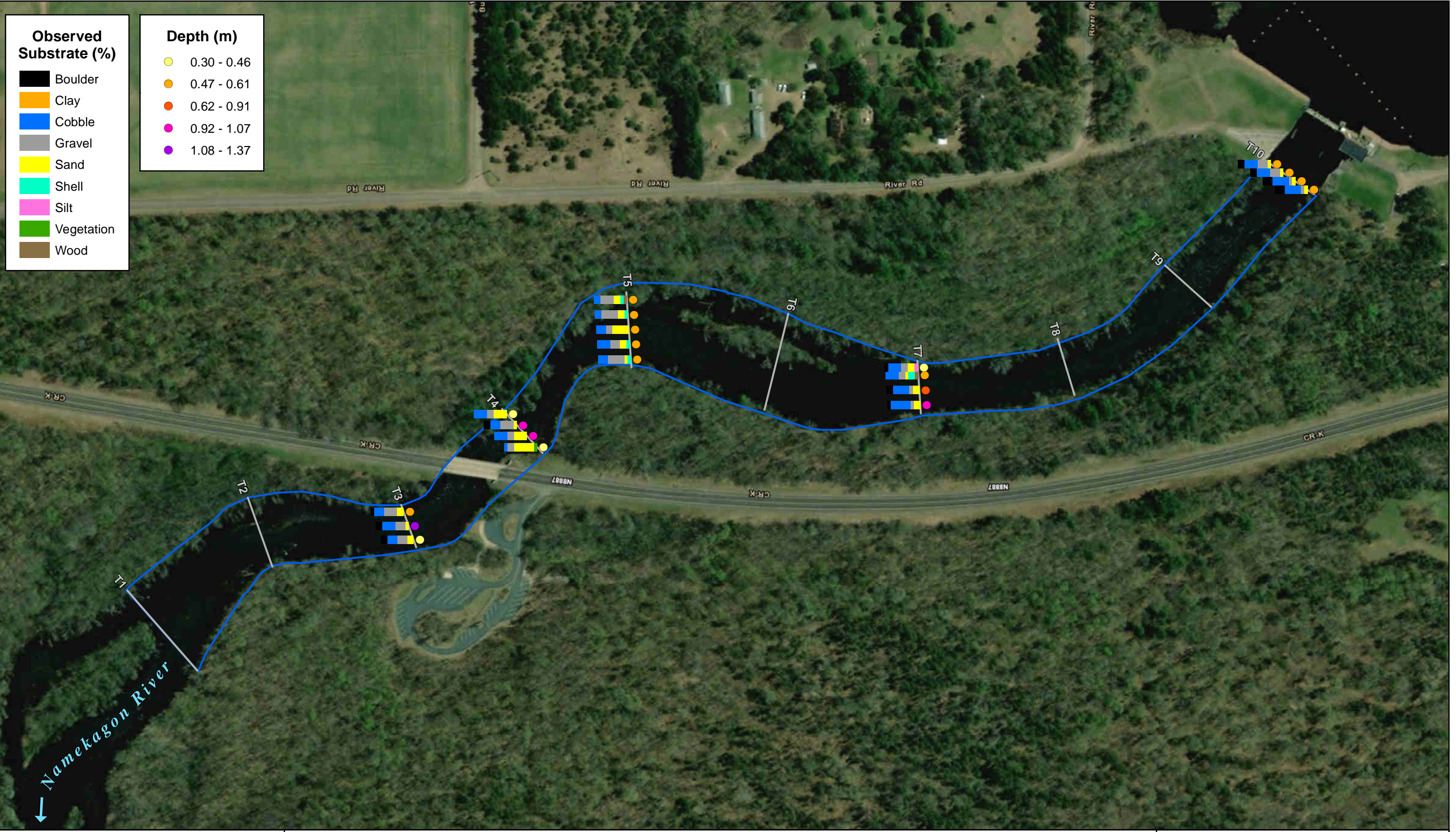
Figure 5. Substrate and Depth for the Trego Project Reach Two on the Namekagon River. Washburn County, Wisconsin.
